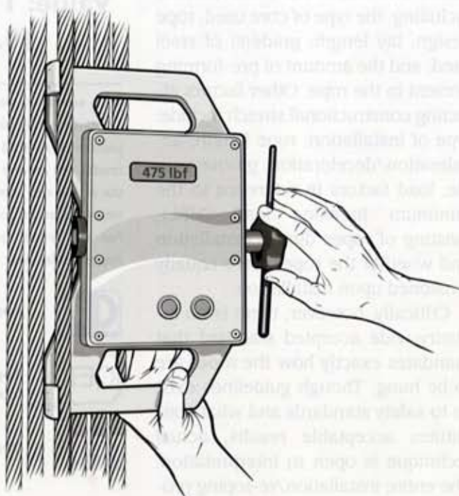
Figure 1: A Brugg Rope Performance Measurement device, an early example of rope measurement. This and its counterparts suffer from an inherent inaccuracy due to a flawed premise for measurement.
