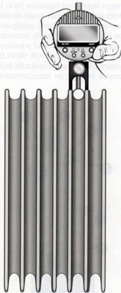
Figure 3: The Brugg GDC allows quick measurement and comparison of sheave groove variations within the sheave itself.
